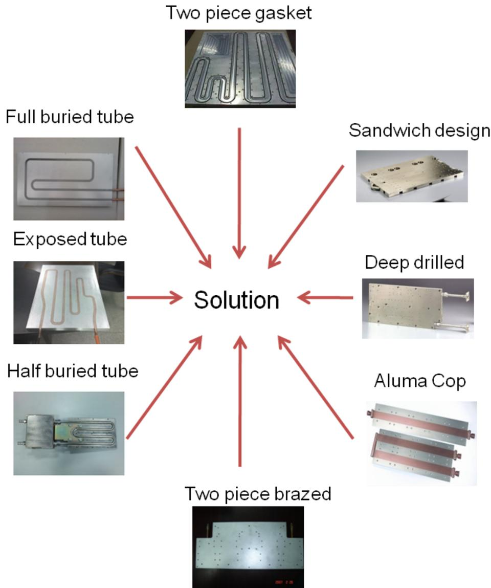
Liquid cold plates can be generally classified into two types, those using a discrete tubing assembly for the liquid pathway and those which have an internal fluid pathway construction.
